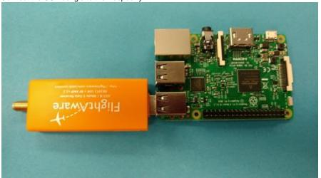
3. Connect the Antenna to the USB dongle
