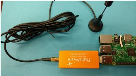
4. Place the Antenna in a location that gives it a clear view of the sky to receive the radio waves
