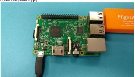
You should observe a solid red LED and a blinking green LED on the Raspberry Pi as well as yellow and green LEDs next to the Ethernet jack.
