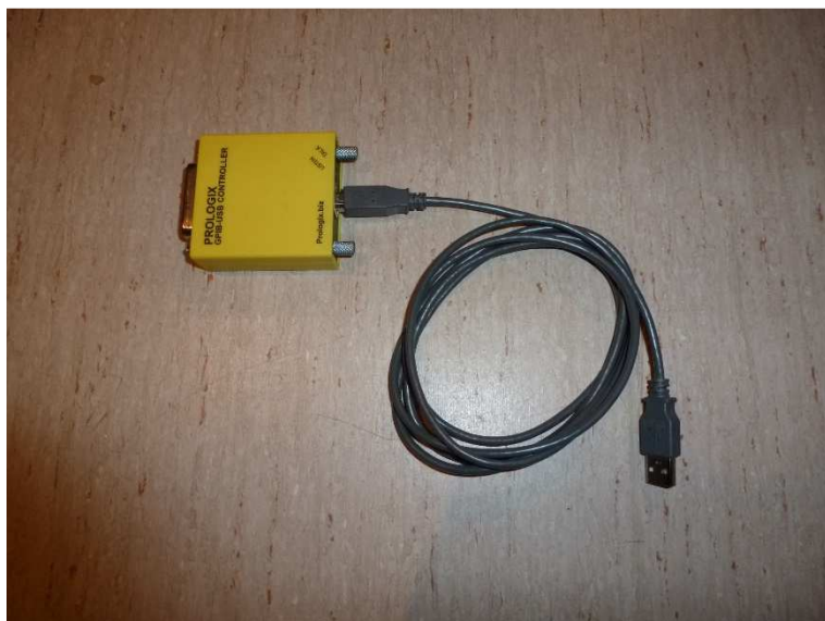
Fig. 19 : Interface GPIB-USB de Prologix, LLC.
